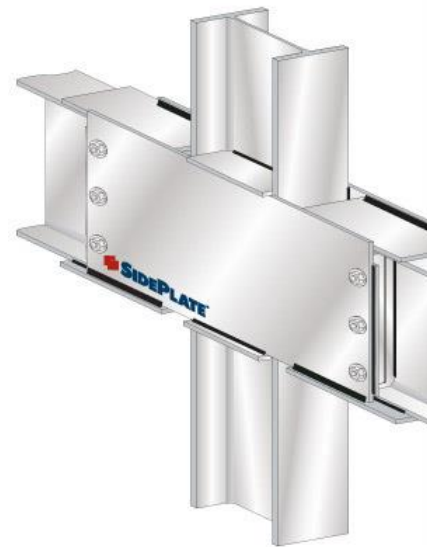
FIGURE S.13: SIDEPLATE CONNECTION (COURTESY OF SIDEPLATE)
